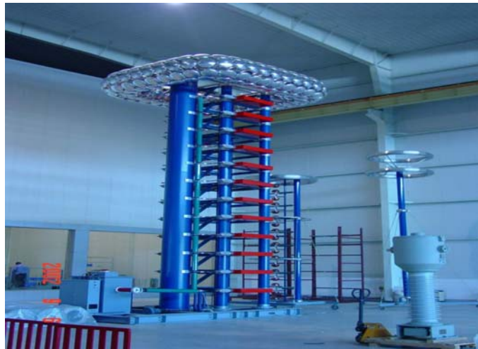
Figure.4 Practical high voltage impulse generator
