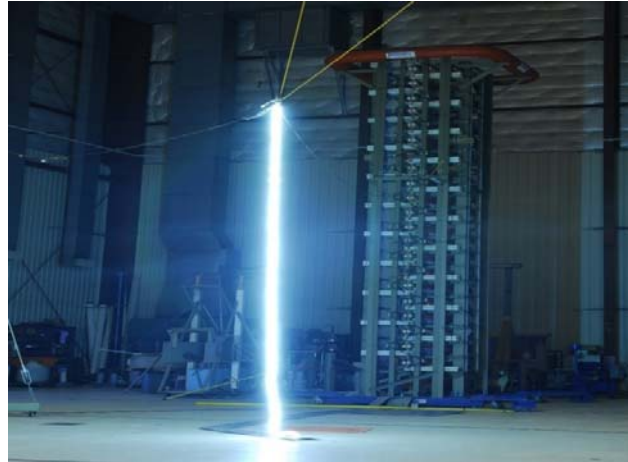
Figure.5 Practical impulse generation for testing
